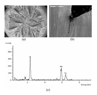
**Fig.7.** SEM (a)Fractured surface of BC 4149, (b)Minor cracks along the inclusion, and (c)MnS.
