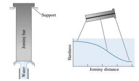
Fig. 2. The Jominy end-quench test.
