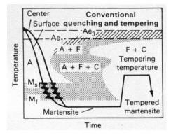
Fig.3. Quench and temper sequence.
