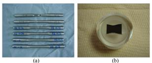
**Fig.11.** (a) Test-pieces with different elongation %, and (b) Metallurgical sample of 17% testpiece.
