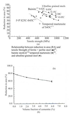
**Fig.10.** (a)Percentage reduction of area with different microstructures, and (b)Reduction of area under different volume of  $2^{nd}$  phase.
