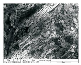
Fig.6. TEM microstructure of BC 4149, tempered at 600°C.
