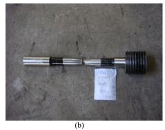
**Fig.9.** (a)A machined test-piece in ISO 898.1 specification, and (b)A machined test-piece from stud.
