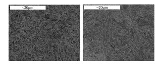
Fig.5. SEM microstructure of BC 4149 (a) 500°C and (b) 600°C .
