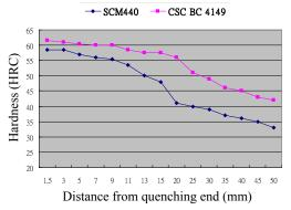
**Fig.4.** Jominy end-quench test result of SCM440 and BC 4149.
